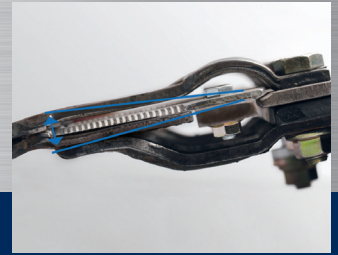
Lacking proper control and guidance, the section wobbles as it moves in the gap, and the wear of all components increases.
