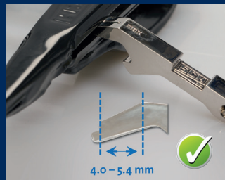
Opening dimension new: 4.0 mm. The control wedge of the MultiTool does not fit into the gap yet.
