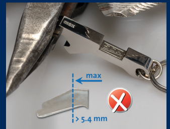
Opening dimension > 5.4 mm: If the control wedge fits completely into the widened gap, the guard can no longer guide the knife safely, it floats.
